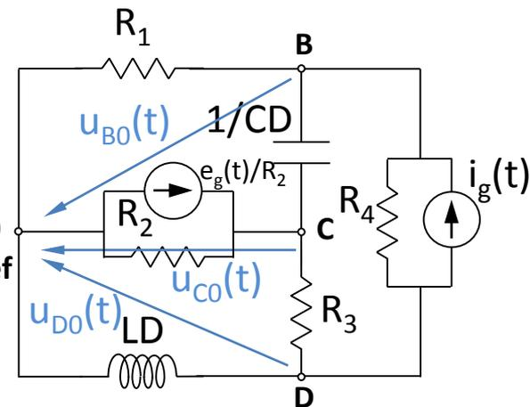
$$\begin{bmatrix} \left( \frac{1}{R_1} + CD + \frac{1}{R_4} \right) & -CD & -\frac{1}{R_4} \\ -CD & \left( \frac{1}{R_3} + CD + \frac{1}{R_2} \right) & -\frac{1}{R_3} \\ -\frac{1}{R_4} & -\frac{1}{R_3} & \left( \frac{1}{R_3} + \frac{1}{LD} + \frac{1}{R_4} \right) \end{bmatrix} \cdot \begin{bmatrix} u_{B0}(t) \\ u_{C0}(t) \\ u_{D0}(t) \end{bmatrix} = \begin{bmatrix} i_g(t) \\ e_g(t)/R_2 \\ -i_g(t) \end{bmatrix}$$
