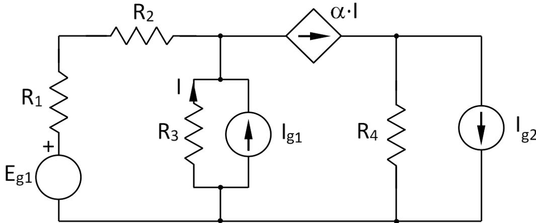
$$R_1 = 1 \Omega, R_2 = 1 \Omega, R_3 = 2 \Omega, R_4 = 2 \Omega, \\ E_{g1} = 4 \text{ V}, I_{g1} = 3 \text{ A}, I_{g2} = 12 \text{ A}, \alpha = 3.$$
