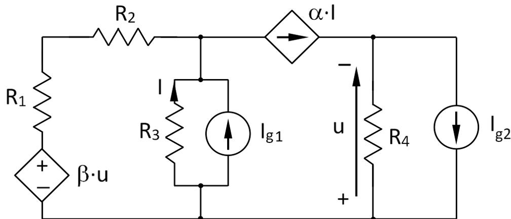
$$R_1 = 1 \Omega, R_2 = 1 \Omega, R_3 = 2 \Omega, R_4 = 2 \Omega, \\ I_{g1} = 3 \text{ A}, I_{g2} = 12 \text{ A}, \alpha = 3, \beta = 1$$
