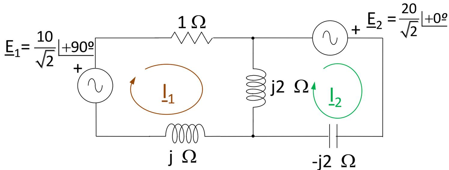
$$\begin{pmatrix} 1 + j2 + j & -j2 \\ -j2 & j2 - j2 \end{pmatrix} \cdot \begin{pmatrix} I_1 \\ I_2 \end{pmatrix} = \begin{pmatrix} \frac{10}{\sqrt{2}}j \\ 20 \\ \frac{20}{\sqrt{2}} \end{pmatrix} \qquad \begin{pmatrix} 1 + j3 & -j2 \\ -j2 & 0 \end{pmatrix} \cdot \begin{pmatrix} I_1 \\ I_2 \end{pmatrix} = \begin{pmatrix} \frac{10}{\sqrt{2}}j \\ 20 \\ \frac{20}{\sqrt{2}} \end{pmatrix}$$
