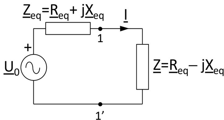
$$\underline{Z}_T = \underline{Z}_{eq} + \underline{Z} = R_{eq} + jX_{eq} + R_{eq} - jX_{eq} = 2R_{eq}$$
