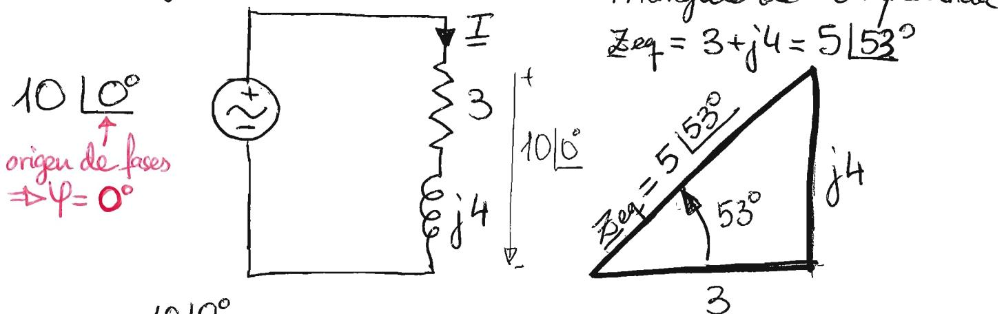
$$I = \frac{10 \angle 0^\circ}{5 \angle 53^\circ} = 2 \angle -53^\circ$$
